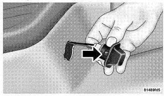
2. Rotate the socket 1/4-turn counterclockwise.
